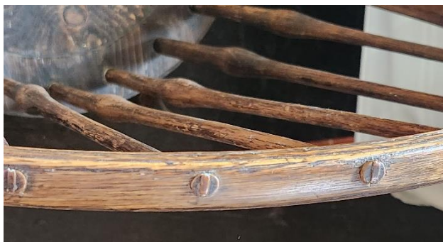
Round-tenoned Spindles pushed into steam bent arched back
